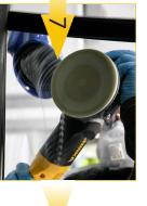
Action: Keep the felt Polishing pad clean to avoid polish build up resulting in a poor finish.
