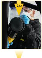
Action: Further reduce scracthes and repair edge. Expand the repair area with finer Abralon discs.
